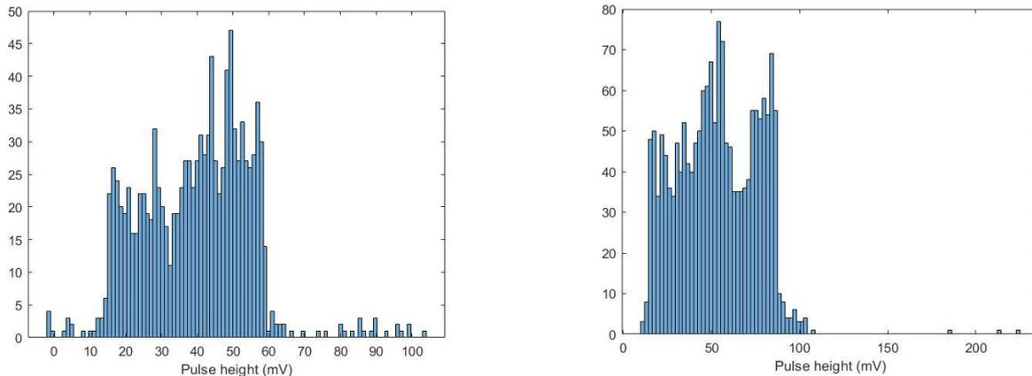
*Legend: histograms of alpha particle events recorded in our instrument during the first two hours after sampling (on the right) and 1 day after (on the left). In abscissa, pulse height is the analogic signal recorded by the instrument, it is equivalent to the energy deposited in the detector by the alpha particle.*
