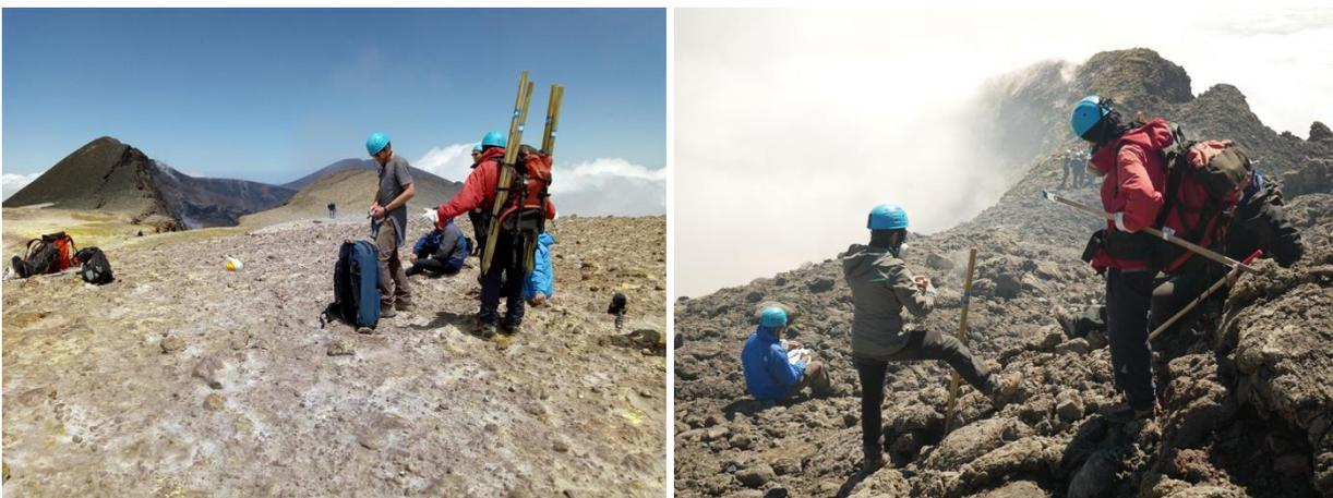
Legend: transport and installation of the radon dosimeters on wood sticks around Etna central crater.
