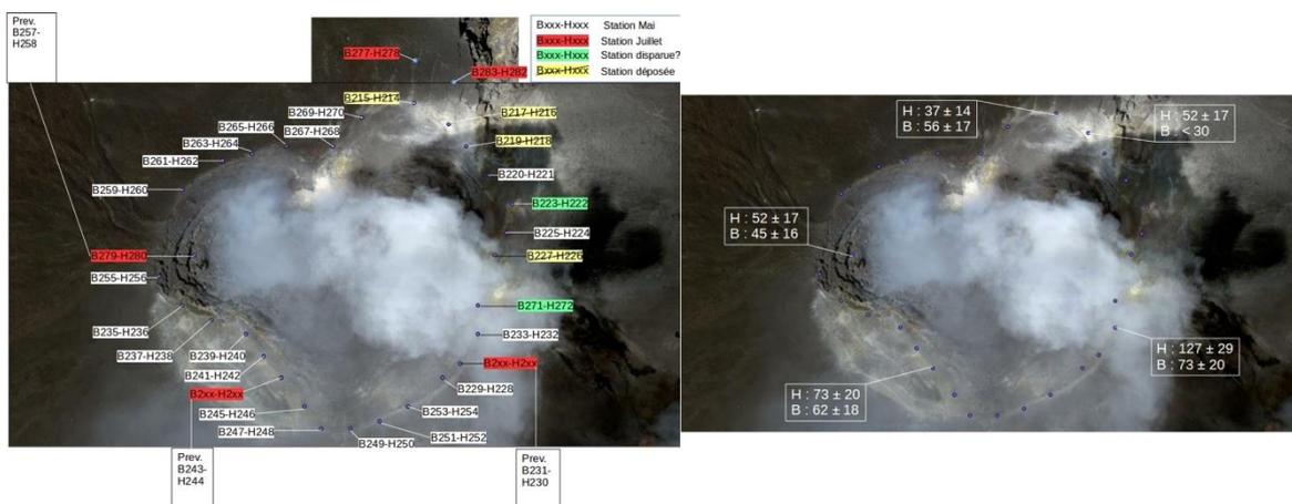
Legend: location of the dosimeters installed in May (left) and first measurements from radon dosimeters collected in July 2018 by Luca Terray (right)
