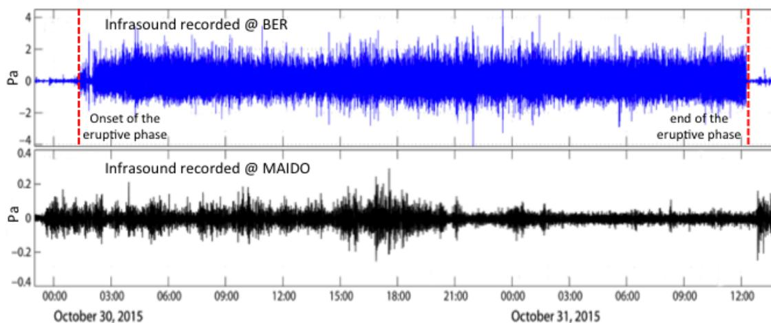
Fig.1 a) infrasonic signal recorded at BER (2.5 km far from the eruptive vent) during the phase 3 (Oct. 30 to Oct. 31) of the 2015 eruption. b) infrasonic signal recorded at MAIDO Observatory (38 km far from the source) during the same period.
