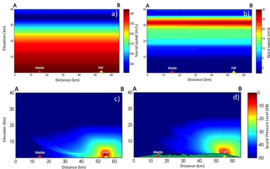
Fig.3 a) Sound speed profile along the section between the two stations. b) Wind speed profile. c-d) Distributions along the section of relative sound pressure level (in decibel) with respect to values at BER without and with topography.
